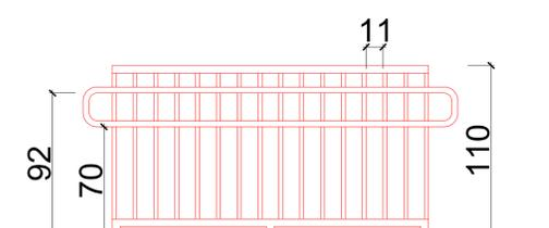
DETALHE GUARDA-CORPO COM CORRIMÃO PARA RAMPAS
